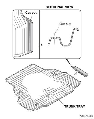
2. Open the trunk lid. Place the trunk tray on the trunk floor.
